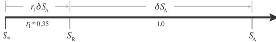
Figure A.4.1. Number line of salinity, illustrating the differences between Preformed Salinity S_* , Reference Salinity S_R , and Absolute Salinity S_A for seawater whose composition differs from that of Standard Seawater.
